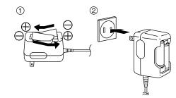
After recharging (about 2 hours), install the charged batteries into the unit.
